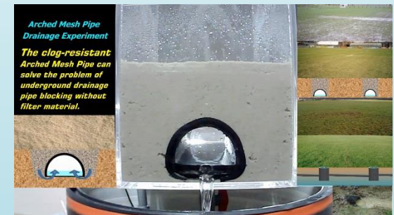
SMPS-Arched Mesh Pipe System Subsurface Drainage Experiment
